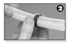
**Step 2.** Slide the correct size crimp ring over the tubing and approximately 2" past the end of the tubing.
