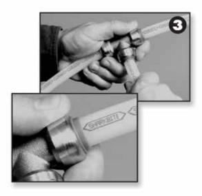
**Step 3.** Insert the tube into the fitting until the tube reaches the tube stop. Make sure the pointed end of the SharkBite pattern is even with the end of the release collar. Only when the tube reaches the tube stop has a secure joint been created.
