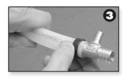
**Step 3.** Push the tubing onto the barbed fitting until it touches the fitting shoulder. Position the crimp ring 1/8"-1/4" from the end of the tube. This distance ensures that the clamp ring is positioned directly over the barbs on the fitting.
