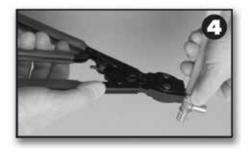
**Step 4.** Position the open jaws of the clamp tool over the raised tabs of the clamp ring and squeeze.
