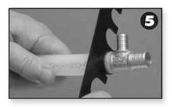
**Step 5.** Verify that the connection is secure by using the go/no-go gauge. The gauge slot that corresponds to the crimp ring size should easily slide onto the compressed crimp ring.
