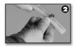
**Step 2.** Slide the correct size clamp ring over the tube and approximately 2" past the end of the tubing.
