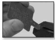
2. Gauge must stop at the NO-GO line in order to make proper connections
