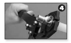
**Step 4.** Position the open jaws of the crimp tool over the crimp ring and squeeze. The jaws are interchangable, and include sizes for 3/8", 1/2", 5/8", 3/4" and 1" crimp rings.
