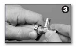
**Step 3.** Push the tubing onto the barbed fitting until it touches the fitting shoulder. Position the clamp ring 1/8"-1/4" from the end of the tube. This distance ensures that the clamp ring is positioned directly over the barbs on the fitting.
